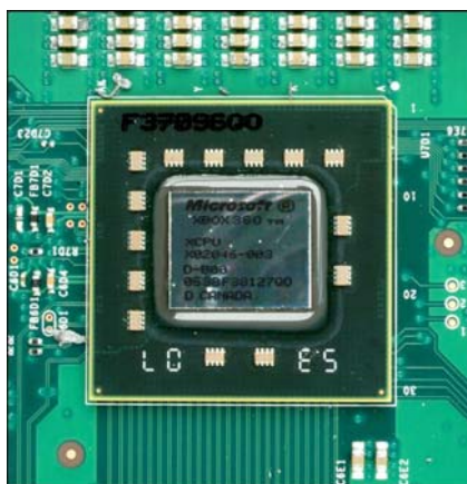
IBM Microelectronics/MS CPU -- in package Part No. X02046-003 Source: Portelligent (die size 12.2mm x 14.8mm)
